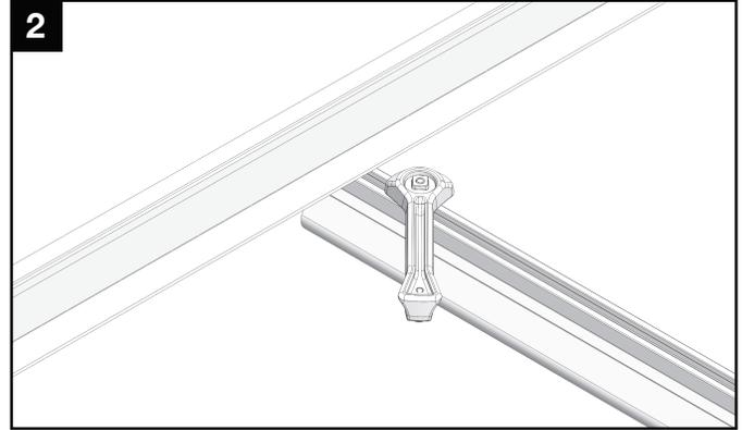
Place module on rails (module cells not shown for clarity).
