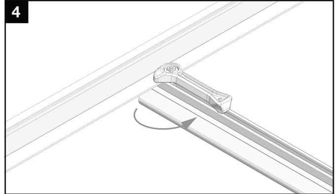
Rotate handle with an upwards motion until CAMO snaps into rail channel. Ensure Camo bonding pins are fully seated on top of module frame.
