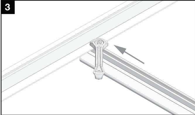
Pull CAMO towards rail ends, at 45 deg angle, so the bonding bolt contacts the module flange edge.
